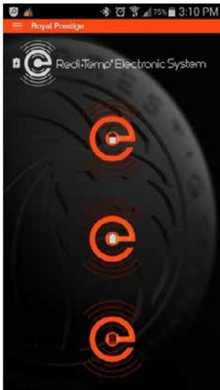
When the temperature of the air passing thru the e-Valves reaches a factory preset point, the e-Valves will automatically turn on, the icon in the center of the e-Valves will illuminate and corresponding icons will appear on the Ready screen. In this illustration, there are three e-Valves that have passed the factory preset on/off point. The e-System can display up to nine (9) active e-Valves.
